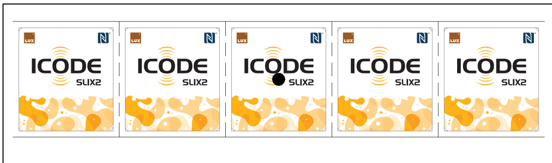
Figure 6: Marking of non-functional RFID labels
